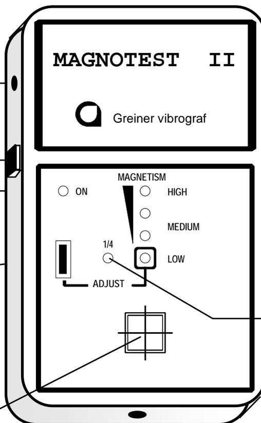
Press and it will divide the reading by 4. Use when object has strong magnetic reading
